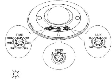
**Note: when testing in daylight, please turn LUX knob to (SUN) position, otherwise the sensor lamp could not work!**
